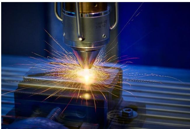
Image 3: High-productivity 3D printing has been made possible by using EHLA technology in a parallel kinematic system and in a modified 5-axis CNC prototype. With the parallel kinematics, for example, the first components made of 316L stainless steel could be printed quickly and reliably at 1.7 kg/h and at a feed rate of 40 m/min. © Fraunhofer ILT, Aachen, Germany.
